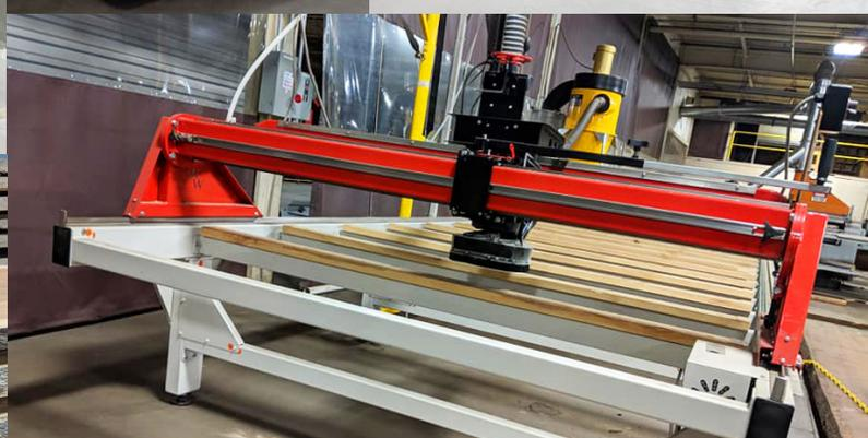
Our WoodWizz tabletop leveler accommodates slabs up to 17' long & 70" wide. Slabs are then sanded (60-120 grit). A slab can typically be completed after 4-6 hours.
